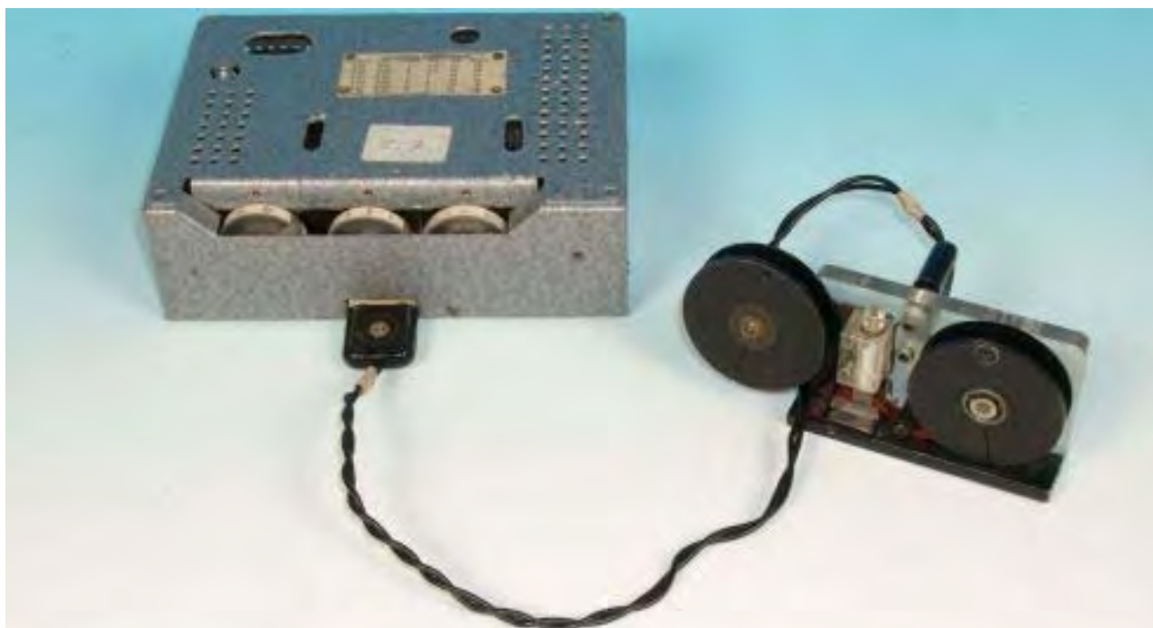
Illustration 13 Old SW transmitter with burst encoder (scanning of a punched tape)
