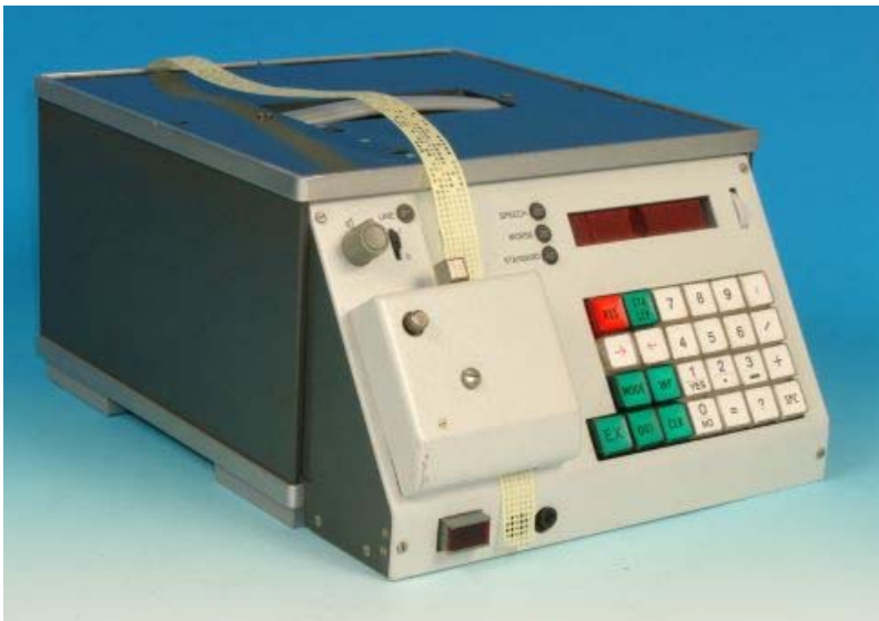
Illustration 06 Speech-Morse generator for the modulation of a SW transmitter. It can be programmed via keyboard, punched tape or computer interface. It is labeled in English since it was delivered to several "Bruderorgane" (brother states' agencies).
