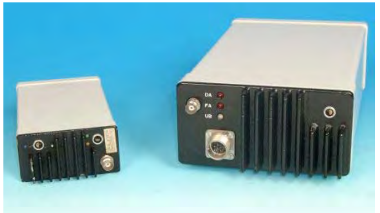
Illustration 22 TSS-2 (transmitter) right, TSE-2 (receiver) left
