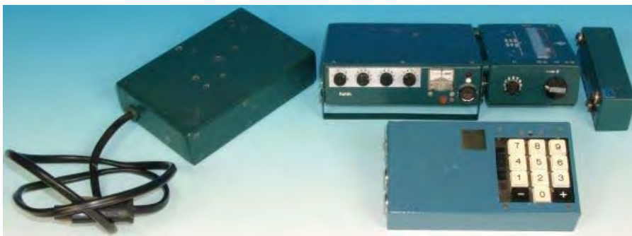
Illustration 16 WSA 1 with power supply unit, antenna matcher and electronic fast coding device
